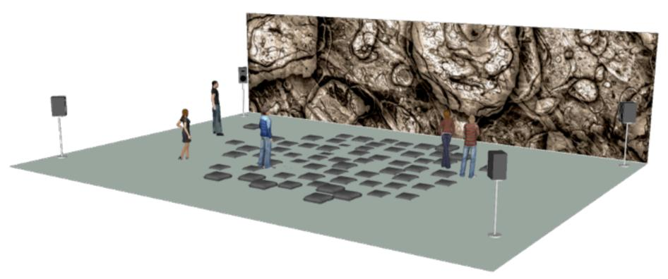
PLASM real-time generative soundscape is encoded in Ambisonics and diffused through a quadraphonic (4.1) sound system. 4 full-range audio signals are fed to the amplifiers. Internal crossover at P.A. level is required to split the frequency range and address the subwoofer. If speakers are full-range and able to play as low as 40 Hz then no subwoofer is required.
